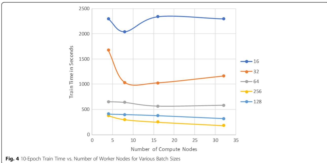
**Fig. 4** 10-Epoch Train Time vs. Number of Worker Nodes for Various Batch Sizes
