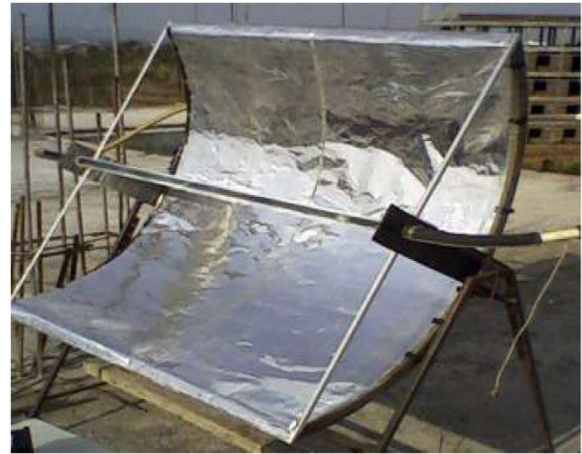
Figure 1 The fiberglass-reinforced plastic parabolic trough.
