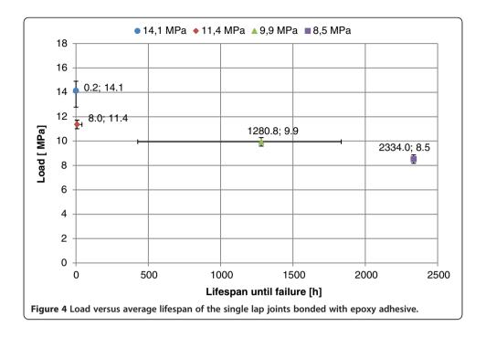
Equation 3 presents the relation between the load and lifespan of the joint using the epoxy based adhesive.
