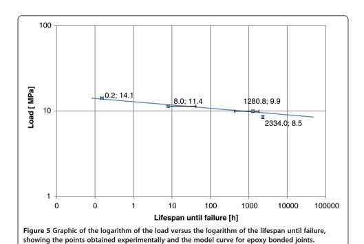
Figure 5 shows the curve governed by Equation 3. It is possible to see that the proposed model is a fair approximation when compared to the experimental data, and that the model curve overlaps along the tolerances of each experimental point. Figure 6 allows us to evaluate the behavior of the joints on a Cartesian scale.
