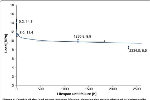
**Figure 6** Graphic of the load versus average lifespan, showing the points obtained experimentally and the model curve in Cartesian scale for epoxy bonded joints.
