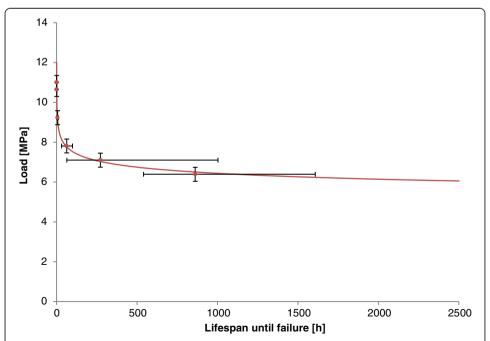
Figure 9 Graphic of the load versus average lifespan, showing the points obtained experimentally and the model curve in Cartesian scale for polyurethane bonded joints.
