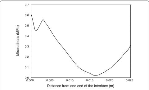
Figure 7 Stress distribution at the interface of the adhesive joint of a riser piper under bending in deep water.
