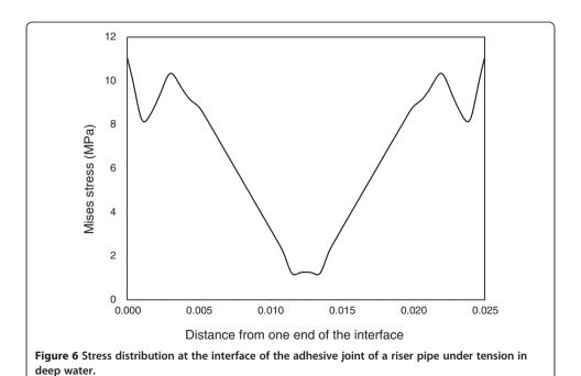
with the element sizes in this paper, which indicates that a singular stress field exists at the end of the interface.
