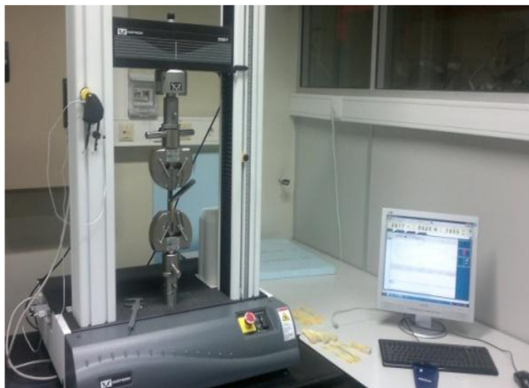
Figure 4 Testing machine and mounting system.
