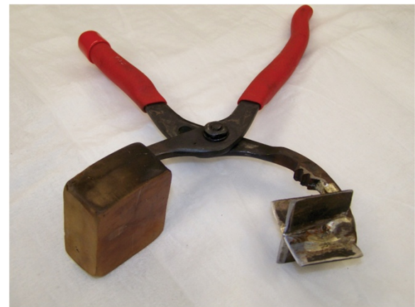
Figure 2 Photograph of the device used to create the liver injury. The stellate shape is as described by Holcomb [37].
