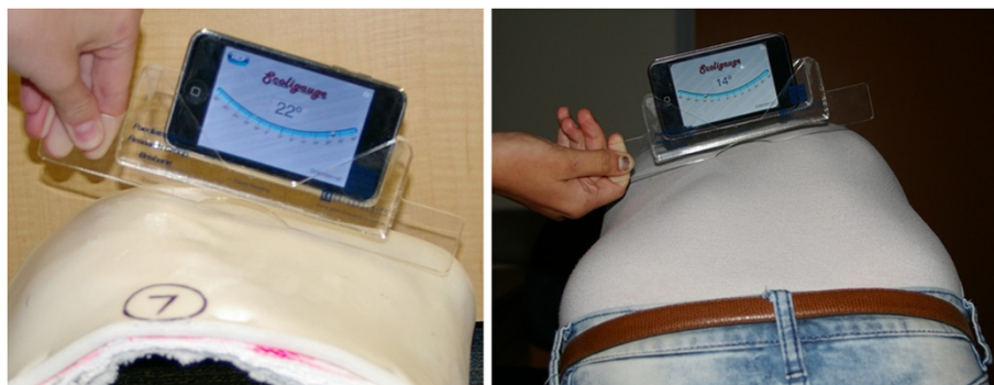
Figure 3 Measurement of the rib hump on a (a) plaster model and a (b) scoliosis patient, using the iPhone and Scoliguage software in combination with the acrylic sleeve to reflect the dimensions of the traditional Scolimeter.
