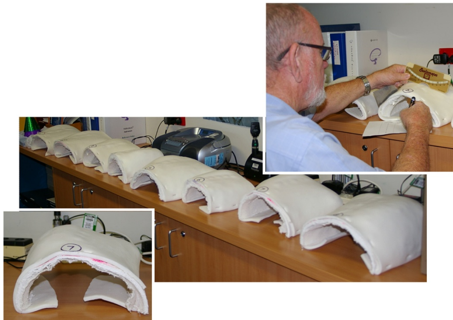
Figure 2 Plaster moulds of eight scoliosis patient's rib humps arranged in random order on a standard height bench in preparation for measurement by each observer with either the Scolimeter or iPhone.
