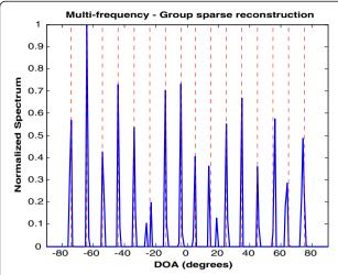
**Figure 16 Multi-frequency group sparse reconstruction.** D = 16 sources with nonproportional spectra.
