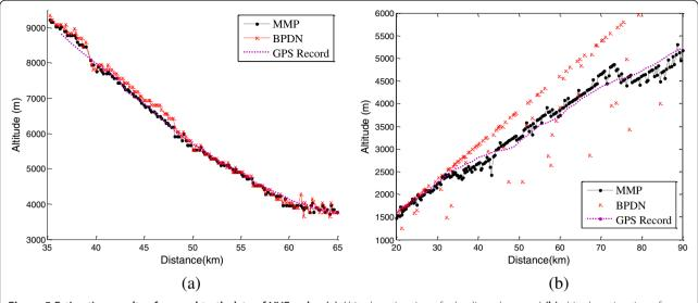
**Figure 5 Estimation results of ground truth data of VHF radar. (a)** Altitude estimation of a landing plane, and **(b)** altitude estimation of a plane taking off.
