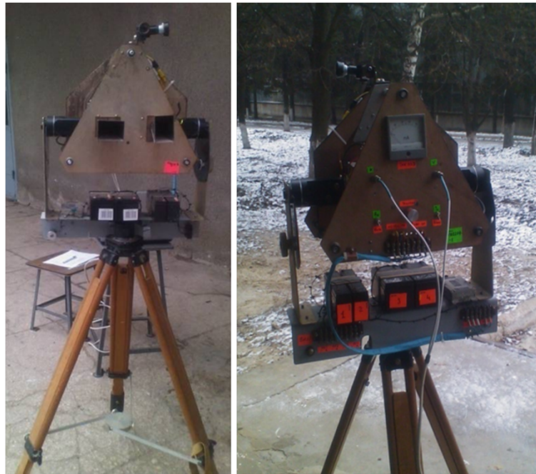
Figure 2 Ground surveillance radar system used for experimental data collection. Wavelength—8.8 mm, emitted radar power—15 mW; receiving/transmitting antenna beam width in both E and H planes—60°; level of side lobes in horn antenna pattern—24 dB; cross-polarization level \leq -30 dB; receiver noise figure—20.2 dB; two-channel 16 bit ADC; and sampling rate in digital records—8 KHz.
