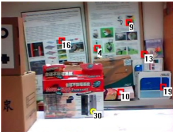
Figure 26 615th frame: feature 30 on the object is detected and initialized with large image depth uncertainty.
