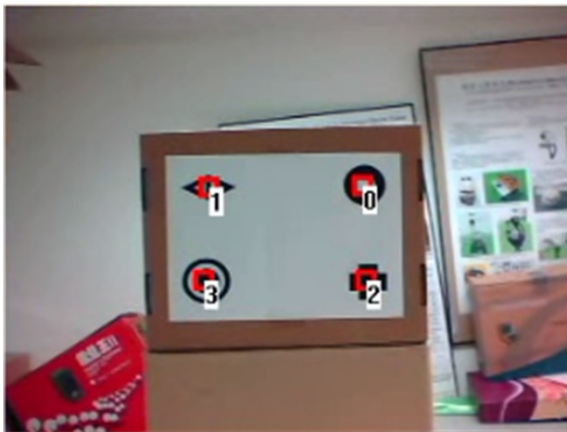
Figure 21 52nd frame: system start-up with four known features, 0, 1, 2, 3.
