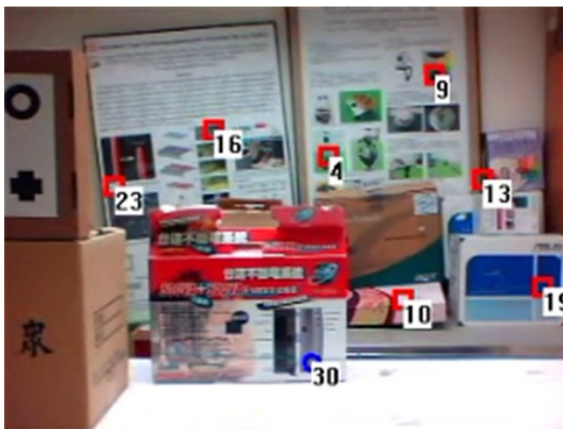
Figure 27 621st frame: the object stops moving and the image depth uncertainty of the feature is reduced.
