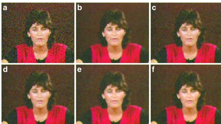
Figure 10 The filtered 10th frames of the Miss America video sequence. (a) Frame corrupted by Gaussian noise, VAR = 0.005, (b) FDMRTF_G, (c) FLRSTF, (d) FLRSTF_ANGLE, (e) VGDF_G, and (f) VMMKNN_G.
