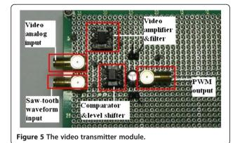
signal, which generates the naturally sampled PWM signal that drives a 5 × 5 red LED cluster. The colors of the LEDs for each signal depend on the transmitted optical power. The semi-angle at half power of the LEDs,  $\theta_{1/2}$ , is 50° (Table 1).
