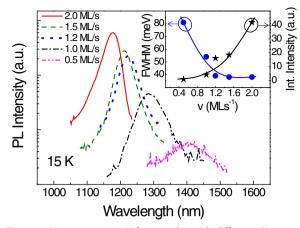
**Figure 3** PL spectra at 15 K for samples with different CL growth rates. The inset shows the FWHM and the integrated intensity as a function of the CL growth rate. Lines are guides to the eye.
