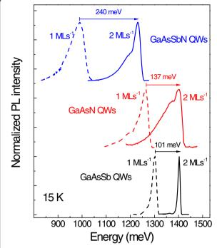
**Figure 5 PL spectra at 15 K for GaAsSb, GaAsN, and GaAsSbN QWs grown at 1 and 2 ML s<sup>-1</sup>.** The spectra corresponding to different materials are shifted in the vertical axis for the sake of clarity. Arrows indicate the respective blueshifts induced by the increased growth rate.
