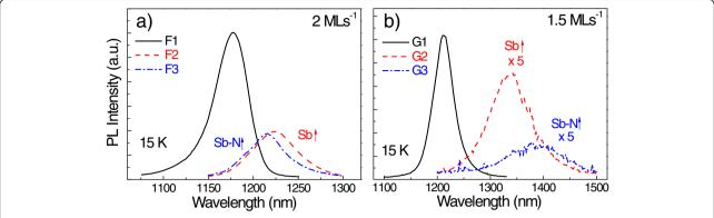
Figure 7 PL spectra at 15 K for samples with different Sb and N contents. PL spectra when increasing the flux of Sb and N during the growth of the CL at (a) 2.0 ML s<sup>-1</sup> and (b) 1.5 ML s<sup>-1</sup>.
