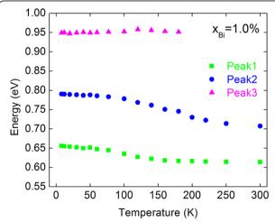
Figure 6 PL energies of the multi-peaks at various temperatures for the InPBi sample with 1.0% Bi. The energy values were extracted by using the multi-peak Gaussian fitting of the PL spectra at various temperatures.
