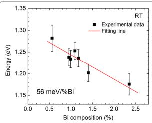
**Figure 3** Bandgap energy of InPBi measured from absorption spectra as a function of Bi composition. The error bars of the experimental data are labeled. The solid line is the fitting line of the experimental data.
