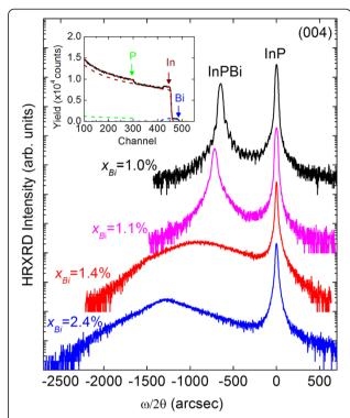
Figure 1 HRXRD (004) scan curves of InPBi samples with various Bi compositions. The inset shows the RBS spectrum from the InPBi film with  $x_{\rm Bi} = 1.4\%$  (solid line). The simulated spectrum and the contributions of Bi, In, P are also contained (dashed lines).
