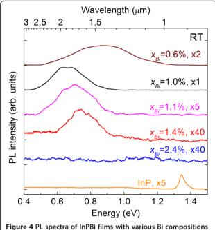
**Figure 4 PL spectra of InPBi films with various Bi composition at RT.** The PL spectrum of InP reference sample is also shown.
