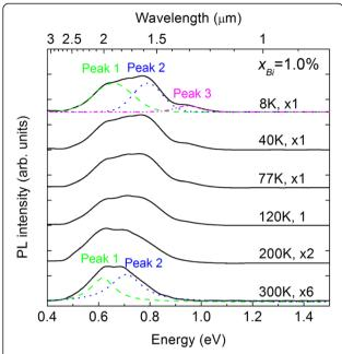
**Figure 5 PL spectra of the InPBi sample with 1.0% Bi at various temperatures.** The overlapped multi-peaks obtained by using Gaussian fitting are shown as the dashed and dotted lines for the cases of 8 and 300 K, and the multi-peaks of PL spectra at other temperatures were also obtained similarly.
