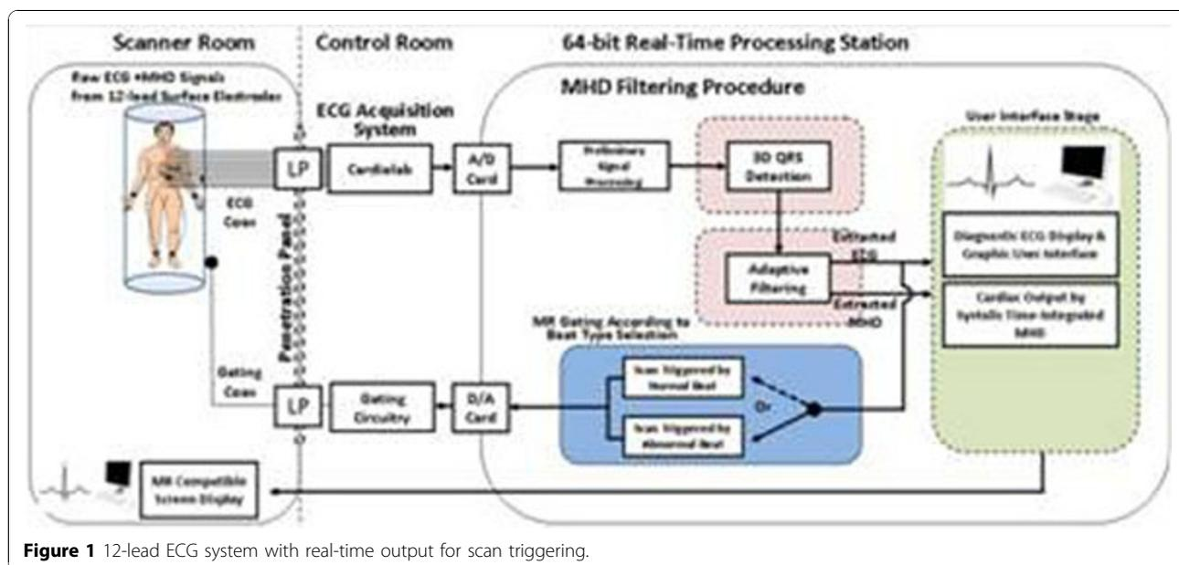
**Figure 1** 12-lead ECG system with real-time output for scan triggering.
