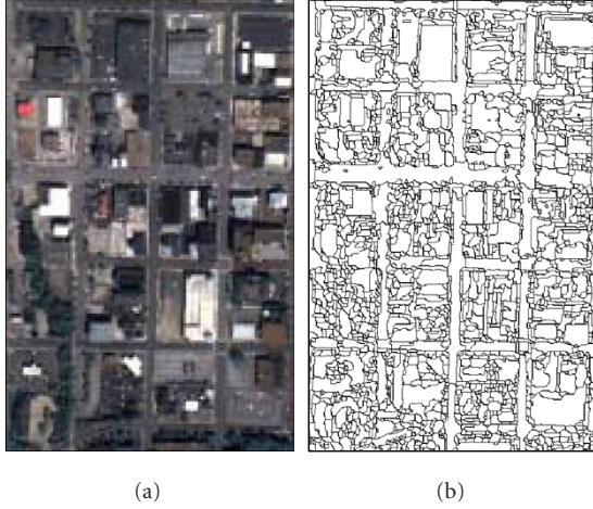
FIGURE 2: (a) A subset of PS-MS IKONOS satellite image in dense urban area of the City of Columbia, Missouri (only R, G, and B channels are shown). (b) Watershed segmentation result.
