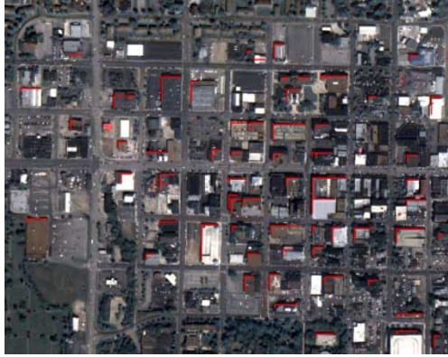
FIGURE 5: Detected shadow corners highlighted in red overlain on the urban area of IKONOS image of City of Columbia, Missouri.
