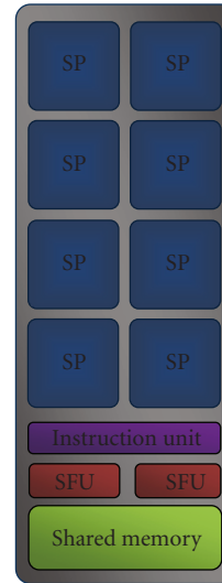
FIGURE 2: Streaming multiprocessors in detail.
