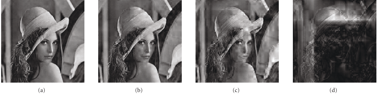
FIGURE 7: The reconstructed images without the 1st, 2nd, 3rd, and 4th layer data, from (a) to (d), respectively.
