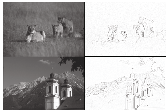
FIGURE 12: Example of the fuzzy contour map obtained for two original images of the Corel database with the Canny filter.
