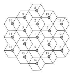
FIGURE 7: HSDPA cell deployment.
