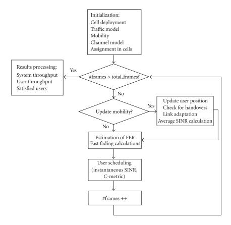
FIGURE 8: System-level simulation procedure flow chart.
