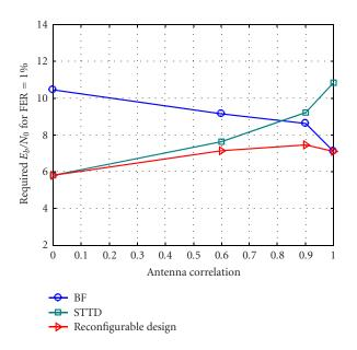
FIGURE 3: Reconfigurability to antenna correlation for two transmit and two receive antennas at 5.4 Mbps.
