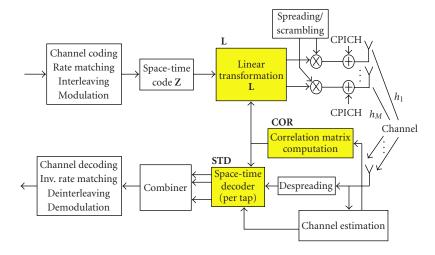
FIGURE 2: Reconfigurability to antenna correlation—transceiver architecture for HSDPA.
