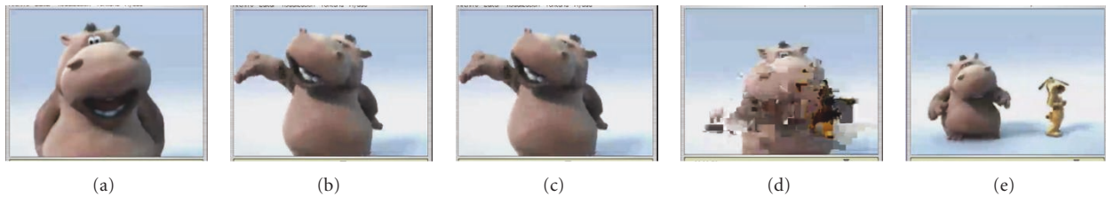
FIGURE 27: Video snapshot: (a) 450 s (before congestion), (b) 470 s (congestion beginning), (c) 480 s (frozen image), (d) 520 s (distortion), and (e) 550 s (recovered image).
