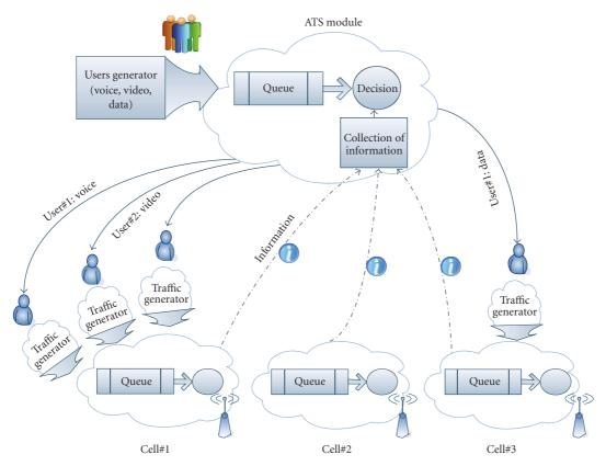
FIGURE 3: General schema representing the different parts of the simulator.
