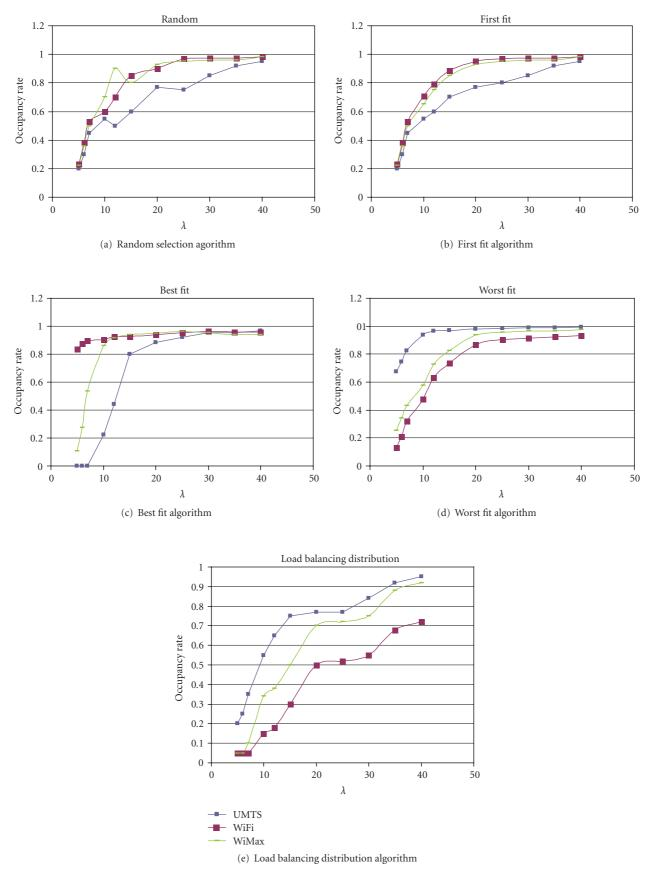
FIGURE 9: Simulation results showing the occupancy rate versus arrival rate.
