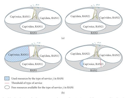
FIGURE 7: (a) Example of the distribution of radio resources on the type of services in two different RANs. (b) When the capacity of "Voice" service exceeds the specified threshold in RAN1, the voice traffic is directed to RAN2.
