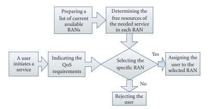
FIGURE 4: Assigning the user to the suitable RAN.
