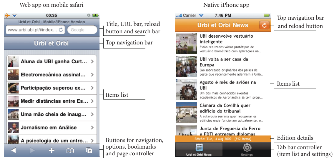
FIGURE 3: Web versus native applications differences and characteristics.
