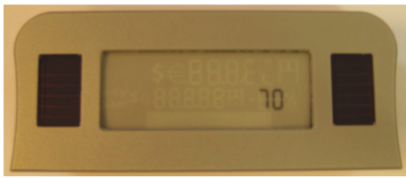
FIGURE 2: Photo of a fully functional energy harvesting electronic shelf label. This label has updated the price (70). We also see the two solar cells on this prototype.
