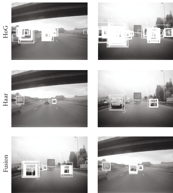
FIGURE 11: Detection results on road (motorway) scene images for three types of detectors.
