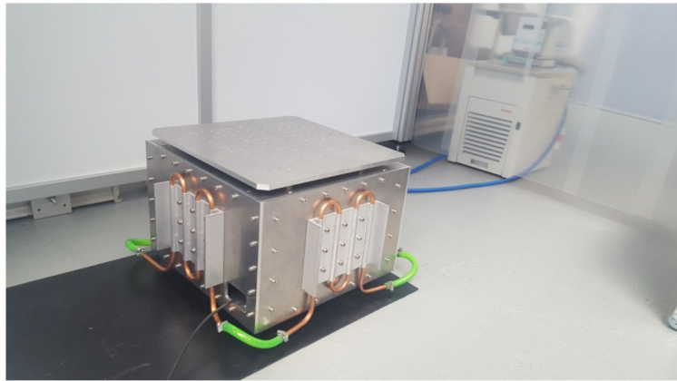
Figure 13 DEPFB device in a cleanroom tent with closed sidewalls and watercooled plates attached to the sides
