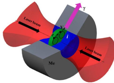
**Fig. 5.** Schematic of laser energy converter into  $\gamma$  radiation.
