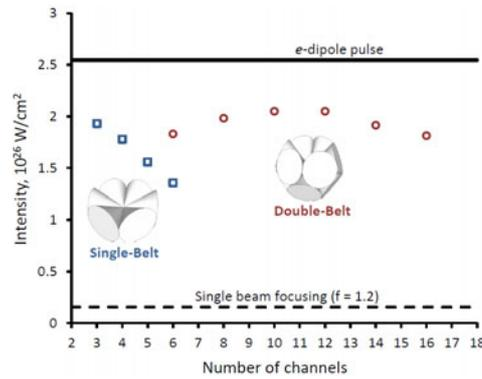
**Fig. 1.** Comparison of belt and double-belt focusing configurations for a different number of laser channels having a total peak power of 200 PW.
