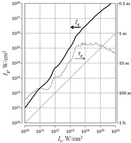
**Fig. 6.** Peak intensity (solid line) and duration (dashed line) of the giant attosecond pulse generated in the case of optimal parameters as a function of the incident wave intensity.
