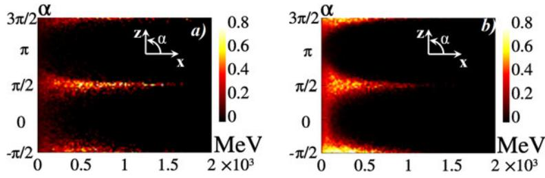
**Fig. 3.** Characteristic photon energy spectrum distribution over angle  $\alpha$  for trajectories in a plane-polarized standing wave a) and in the field of a dipole wave b).
