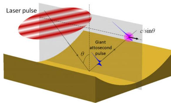
**Fig. 7.** Schematic representation of the concept of groove-shaped target.
