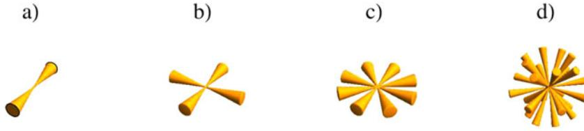
**Fig. 1.** The concept of multi-beam technology: planer setup with a)  $n = 2$ , b)  $n = 4$ , c)  $n = 8$  colliding pulses and 3D setup d) with  $n = 24$  colliding pulses (as proposed in [39]).
