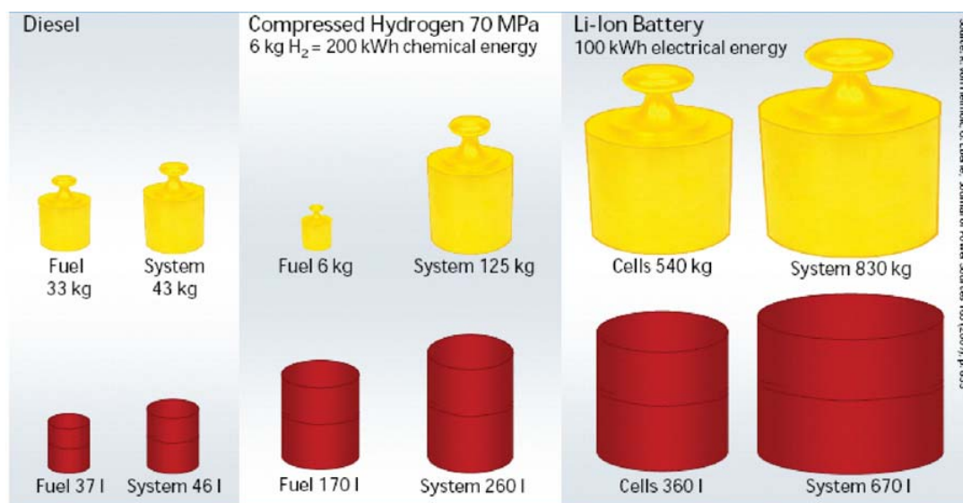
Fig. 1. Comparison of weight and volume of diesel fuel, hydrogen, and a Li-ion battery pack for equivalent driving ranges (from ref. [5]).
