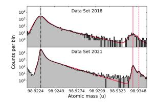
Fig. 5 The discovery of  $^{99m}$ In isomer with recent upgrade in ISOLTRAP's MR-TOF-MS mass-resolving power in 2021 [50]. The issue was not resolved in the 2018 campaign, where the measurement was performed with a lower mass resolution. The red solid and dashed lines show the ground and isomeric state of  $^{99g, m}$ In, respectively. Source: reprinted figure with permission from [50]
