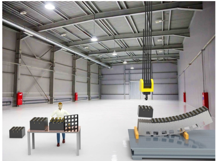
(b) Illustration of the assembly of two PMT mounting boxes by a technician, as well as the mounting of six photo-module boxes into an arch for subsequent mounting on the detector frame (see Fig. 7.7)
