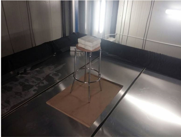
Fig. 3 Photograph of the Pb blocks, with an overall volume of 4\text{ dm}^3 , which were positioned inside the volume defined by the upper and lower trackers
