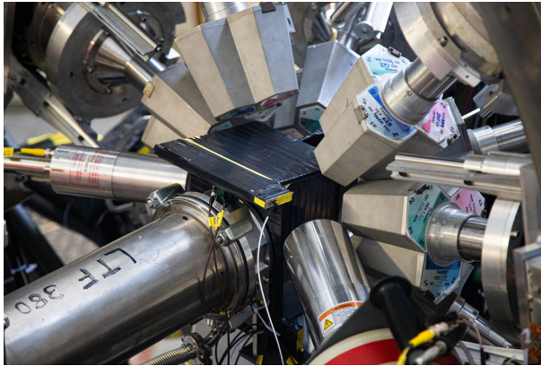
Fig. 10 For the measurement of the ^{226}\text{Ra} and ^{248}\text{Cm} targets, the Miniball germanium detector array [60] was set up in the \pi\text{E1} area
