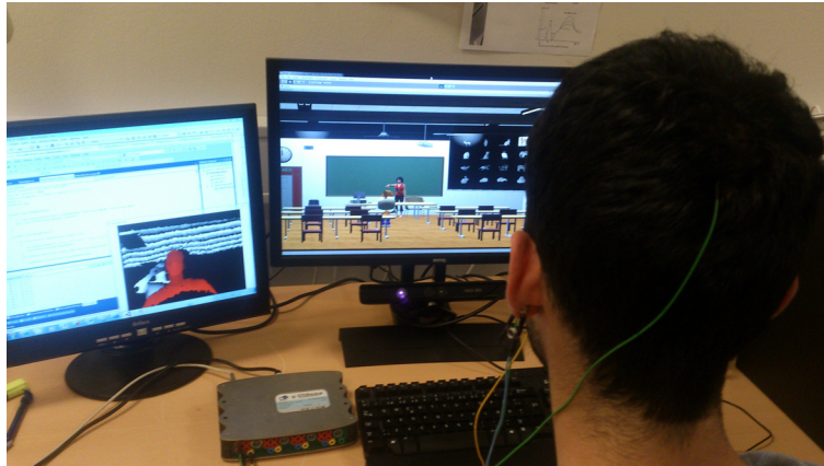
Fig. 4 Illustration of the experimental setup. G.USBamp is seen on the table with the attached EEG electrodes. The reference electrode on the left earlobe and the recording electrode from Pz is visible. The Kinect situated below the interface screen is turned on and tracking the subject. The tracked area is visualized in the left screen as the red area, with the ceiling and the person taking a photo is colored gray representing ignored depth value measurements
