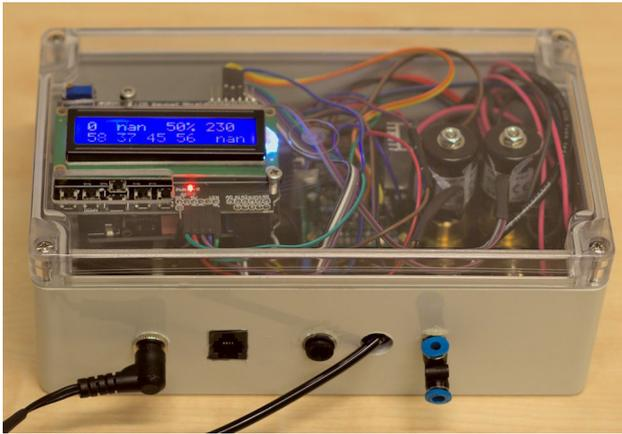
**Fig. 2** Picture of the finished device, excluding the power supply, gas washing bottles, and chamber. The enclosure contains the Arduino microcontroller (with display and keypad mounted in the lid), solenoid valves, electronics (solenoid drivers, temperature monitor, and wiring between all modules). Dimensions:  $200 \times 120 \times 75$  mm
