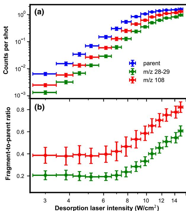
**Fig. 3** Dependence of the cw-LIAD process on desorption laser intensity. **a** Ion yields for adenine parent and selected fragments at different desorption laser intensities. **b** Observed fragment-to-parent ratios as a function of desorption intensity. All data was collected at  $\sim 1.4 \times 10^{13}$   $W/cm^2$  ionisation intensity. Error bars show standard errors
