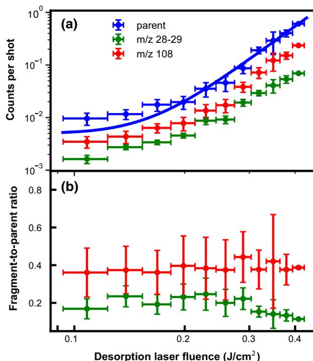
**Fig. 2** Dependence of the ns-LIAD process on desorption laser fluence. **a** Ion yields for adenine parent and selected fragments at different desorption laser fluences, the solid line corresponds to a power-law fit (see text for details). **b** Observed fragment-to-parent ratios as a function of desorption fluence. All data was collected at  $\sim 1.4 \times 10^{13}$  W/cm<sup>2</sup> ionisation intensity. Error bars show standard errors
