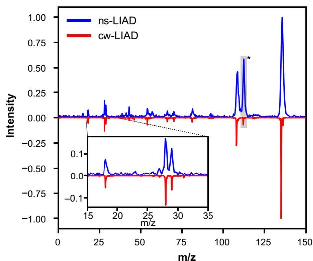
**Fig. 1** Normalised mass spectra of adenine following desorption by ns-LIAD (blue) or cw-LIAD (red), and multiphoton ionisation by 800 nm femtosecond pulses ( $\sim 1.4 \times 10^{13}$  W/cm<sup>2</sup>). The shaded peak marked with an asterisk is due to a background contamination in the vacuum chamber
