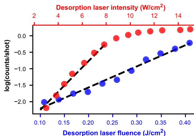
**Fig. 4** Comparison of the observed parent ion signal as a function of desorption laser fluence for ns-LIAD (blue, bottom  $x$ -axis) or intensity for cw-LIAD (red, top  $x$ -axis). The dashed lines are the result of a linear fit to the data and highlight the region where the dependence can be described by a power-law
