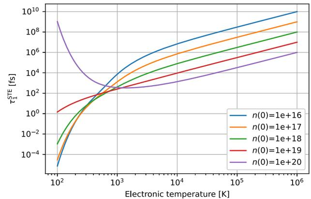
**Fig. 2** Effective STE formation time,  $\tau_1^{\text{ste}}(t)$ , as a function of the electronic temperature,  $T_n$ , for a selection of initial densities,  $n(0)$ . The initial densities  $n(0) = 10^{16}, 10^{17}, 10^{18}$  cm<sup>-3</sup> are below,  $10^{19}$  cm<sup>-3</sup> slightly below and  $10^{20}$  cm<sup>-3</sup> above the EMT, respectively
