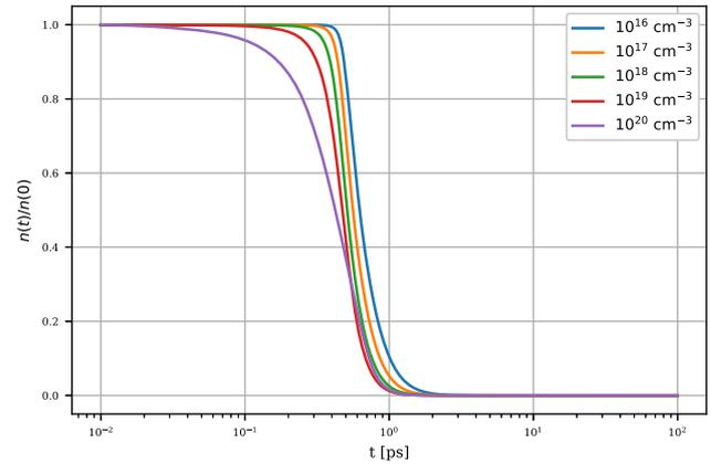
**Fig. 1** Free electron–hole pair density,  $n(t)$ , normalised to the initial density,  $n(0)$ , for a selection of initial densities,  $n(0)$ . The initial densities  $n(0) = 10^{16}, 10^{17}, 10^{18}$  cm<sup>-3</sup> are below,  $10^{19}$  cm<sup>-3</sup> slightly below and  $10^{20}$  cm<sup>-3</sup> above the EMT, respectively
