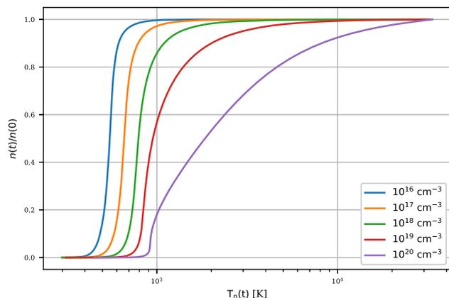
**Fig. 3** Free electron–hole pair density,  $n(t)$ , normalised by the initial density,  $n(0)$ , as a function of the electronic temperature,  $T_n$ , for a selection of the initial density,  $n(0)$ . The initial densities  $n(0) = 10^{16}, 10^{17}, 10^{18} \text{ cm}^{-3}$  are below,  $10^{19} \text{ cm}^{-3}$  slightly below and  $10^{20} \text{ cm}^{-3}$  above the EMT, respectively
