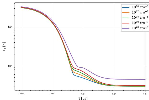
**Fig. 4** Electronic temperature,  $T_n(t)$ , for a selection of the initial density,  $n(0)$ . The initial densities  $n(0) = 10^{16}, 10^{17}, 10^{18} \text{ cm}^{-3}$  are below,  $10^{19} \text{ cm}^{-3}$  slightly below and  $10^{20} \text{ cm}^{-3}$  above the EMT, respectively
