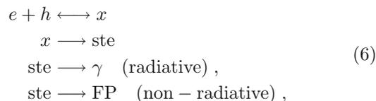
where  $\gamma$  stands for photon and ‘FP’ for Frenkel pair of point defects. The last two reactions give the two STE decay pathways [10]. We initially assume that the STEs cannot ‘untrap’ and postpone the discussion of the thermal detrapping of STEs to the end of Sect. 5. For the sake of simplicity, we also neglect the impact dissociation of STEs.
