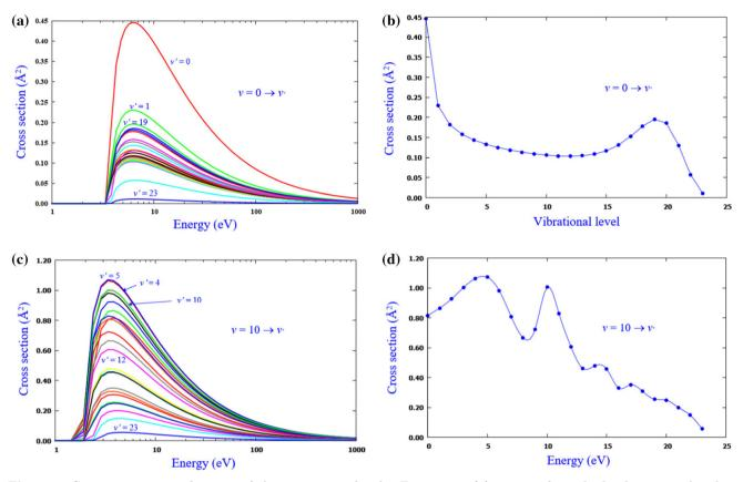
Fig. 1 a Cross sections as a function of electron energy for the E-v process (1) starting from the level v = 0 and ending on all the v' levels (some indicated in the figure). **b** corresponding cross section maxima for the same process as a function of the final vibrational levels v'. Same for the lower frames but for the E-v process starting from v = 10. In the panel (d), the cross section markers were connected by a smoothed line
