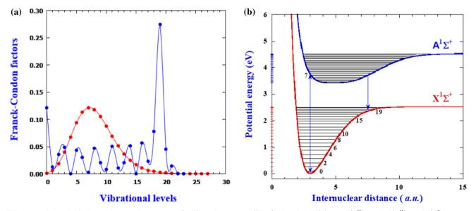
Fig. 2 a Franck–Condon factors for  $q_{v=0,v''}$  (red) and  $q_{v''=7,v'}$  (blue), for the  $X(v) \to A(v'')$  and  $A(v'') \to X(v')$  transitions, respectively. **b** Potential energy curves for the LiH singlet electronic states. The horizontal lines, and the corresponding ticks on the *y*-axis, give the energy position of the vibrational eigenvalues. In the panel (a), the markers of the FC factors were connected by a smoothed line
