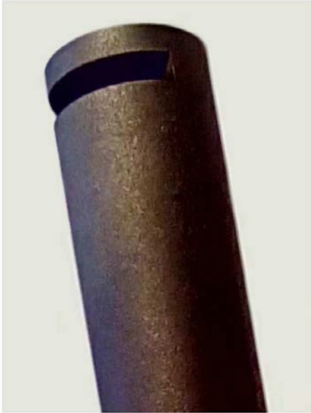
Fig. 6. Bunker Probe (BUP) of graphite (from Costea et al. [28]). The cylindrical piece has an outer diameter of 12 mm and an inner diameter of 8 mm. It is closed on top and has a 2 mm wide slit which encompasses half the cylinder's circumference.
