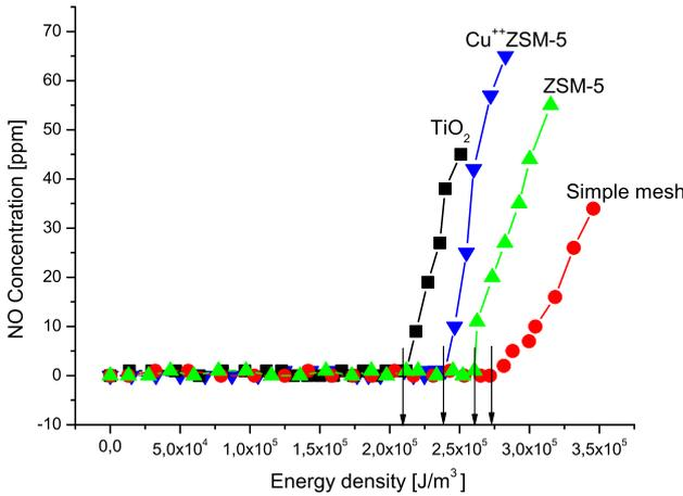
**Fig. 4.** (Color online) Nitrogen monoxide concentration versus energy density for the discharge with the needle to the mesh electrodes; needle to the mesh electrodes with  $\text{TiO}_2$ ; with ZSM-5, or with  $\text{Cu}^{++}\text{ZSM-5}$ . Needle negative,  $d = 8.1$  mm,  $Q = 1.8$  slm,  $RH = 0.8\%$ . Mass of  $\text{TiO}_2$  globules  $m = 0.7691$  g, mass of ZSM-5  $m = 0.5203$  g and mass of  $\text{Cu}^{++}\text{ZSM-5}$   $m = 0.5398$  g.
