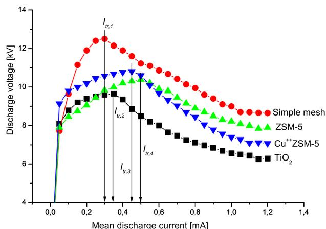
**Fig. 2.** (Color online) Volt-ampere characteristics for the discharge with the needle to the mesh electrodes; needle to the mesh electrodes with  $TiO_2$ ; with ZSM-5, or with  $Cu^{++}$ ZSM-5. Needle negative,  $d = 8.1$  mm,  $Q = 1.8$  slm,  $RH = 0.8\%$ . Mass of  $TiO_2$  globules  $m = 0.7691$  g, mass of ZSM-5  $m = 0.5203$  g, mass of  $Cu^{++}$ ZSM-5  $m = 0.5398$  g.
