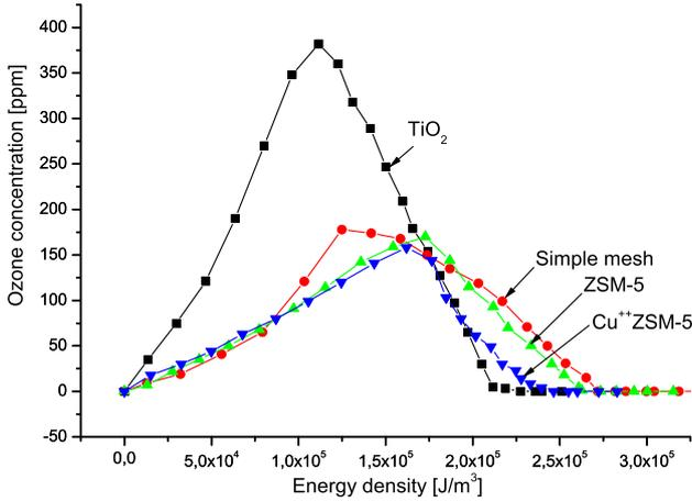
**Fig. 3.** (Color online) Ozone concentration versus energy density for the discharge with the needle to the mesh electrodes; needle to the mesh electrodes with  $\text{TiO}_2$ ; with ZSM-5, or with  $\text{Cu}^{++}\text{ZSM-5}$ . Needle negative,  $d = 8.1$  mm,  $Q = 1.8$  slm,  $RH = 0.8\%$ . Mass of  $\text{TiO}_2$  globules  $m = 0.7691$  g, mass of ZSM-5  $m = 0.5203$  g, mass of  $\text{Cu}^{++}\text{ZSM-5}$   $m = 0.5398$  g.
