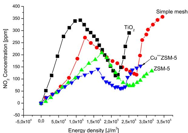
**Fig. 5.** (Color online) Nitrogen dioxide concentration versus energy density for the discharge with the needle to the mesh electrodes; needle to the mesh electrodes with  $\text{TiO}_2$ ; with ZSM-5, or with  $\text{Cu}^{++}\text{ZSM-5}$ . Needle negative,  $d = 8.1$  mm,  $Q = 1.8$  slm.  $RH = 0.8\%$ . Mass of  $\text{TiO}_2$  globules  $m = 0.7691$  g, mass of ZSM-5  $m = 0.5203$  g and mass of  $\text{Cu}^{++}\text{ZSM-5}$   $m = 0.5398$  g.
