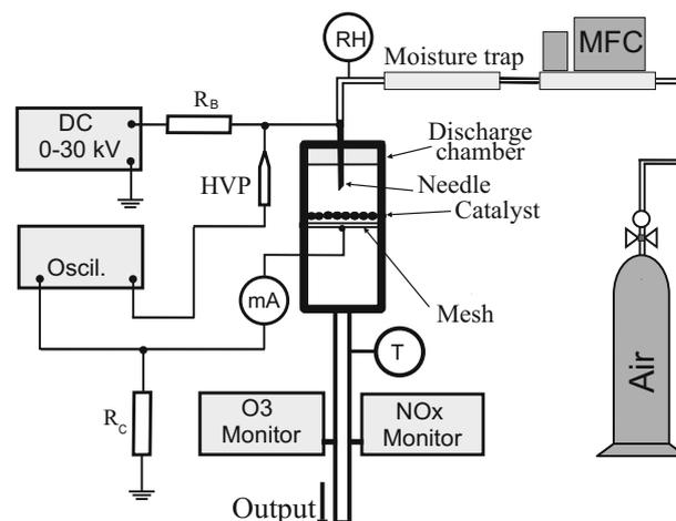
**Fig. 1.** Experimental arrangement. *RH* – relative humidity sensor, *MFC* – mass flow controller, *T* – thermometer,  $R_B$  – ballast resistor,  $R_C$  – earthed resistor.
