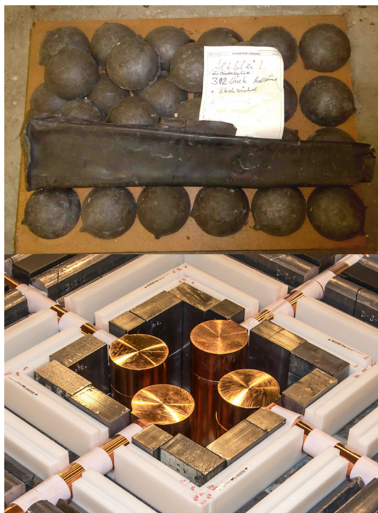
Fig. 15 Top: Old Pb half-spheres from the Freiburg Minster, low in ^{210}\text{Pb} activity. Bottom: Innermost Pb layer of the CONUS shield consisting among others of the Pb bricks melted from the Freiburg Minster Pb
