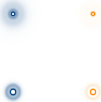
Fig. 10 The radial component of the electric field (left, blue) with e = 1 and the energy density (right, orange) associated to the model in Sect. 4.1.1 depicted in the plane for \sigma = 5 and \alpha = 2 , with k = 1 (top), and k = 2 (bottom). The intensity of the blue and orange colors increases with the increasing of the electric field and energy density, respectively
