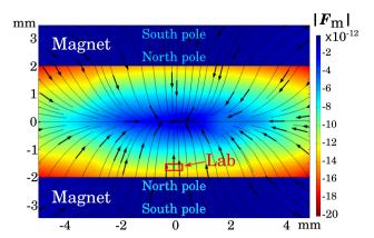
Fig. 16 The magnetic force field of the considered setup for two 1.25 T neodymium magnets, in units of  $10^{-12}$  N. The separation between the two magnets (depicted in dark blue) is 4 mm. The radius of the magnets on the plane parallel to the orbits is 15 mm. The equilibrium position of the Satellite is approximately 300  $\mu$ m above the north pole of the lower magnet. The Lab zone is represented by a red rectangle. We used the COMSOL Multiphysics® software to perform the modeling [45]
