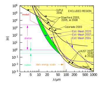
**Fig. 3** Present 95% CL exclusion contours (in yellow) from several experiments on Yukawa-like deviations from Newton's  $1/r^2$  law in the  $(\lambda, |\alpha|)$  plane (from Refs. [16–24]). In green, the region excluded by the recent analysis in Ref. [25]. The figure is adapted from this last reference
