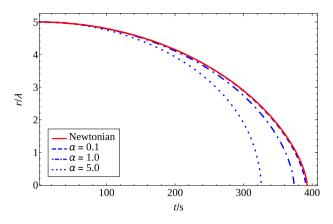
**Fig. 1** Left: normalized distance  $a=r/\lambda$  between the Satellite, S, and the source of the gravitational field, P, as a function of time, in the case of Newtonian (red solid line) and Beyond-Newtonian motion (blue non-solid lines). The initial conditions are  $a_0=5$  and  $\dot{a}_0=0$ , with  $k=G_{\rm N}m_{\rm P}/\lambda^3=10^{-3}~{\rm s}^{-2}$  and  $\lambda=10~{\rm \mu m}$  for different  $\alpha$ :  $\alpha=0.1$
