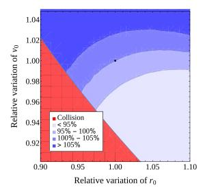
$\rm s^{-1}$  and  $\dot{\theta}_0 = 395.5~\mu \rm rad~s^{-1}$ . Variations which will generate collision are represented in meshed red. We observe that the second set of initial conditions is more "robust" against uncertainties in their fixing
