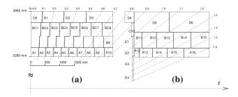
**Fig. 4** The cell structure in the right half the long barrel (a) and extended-barrel (b) module of the calorimeter. The left half of the long barrel is not shown as the long barrel is symmetrical. Solid lines show the cell boundaries formed by grouping optical fibers from the tiles for read out by separate PMTs. The dashed lines represent fixed pseudorapidity values
