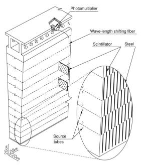
**Fig. 3** Mechanical structure of a TileCal module, showing the slots in the steel for scintillating tiles and the method of light collection by wavelength-shifting fibres to PMTs. The holes for radioactive source tubes that traverse the module perpendicularly to the iron plates and scintillating tiles are also shown
