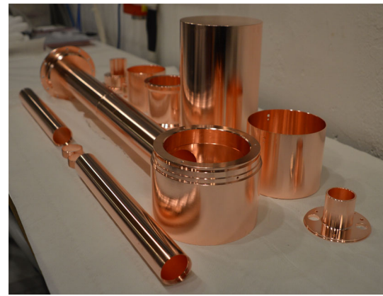
Fig. 5 Electropolished copper cryostat parts used for the construction of the first CONUS detector C1
