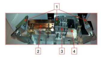
**Fig. 2** The HiRadMat crystal experiment setup: (1) are the three gafcromic foils, (2) is the copper mask, (3) is the STF103 crystal and (4) is the QMP33 crystal
