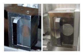
Fig. 3 Picture of the QMP33 crystal before (left) and after (right) the irradiation
