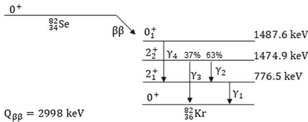
Fig. 1 Decay scheme of <sup>82</sup>Se to <sup>82</sup>Kr
