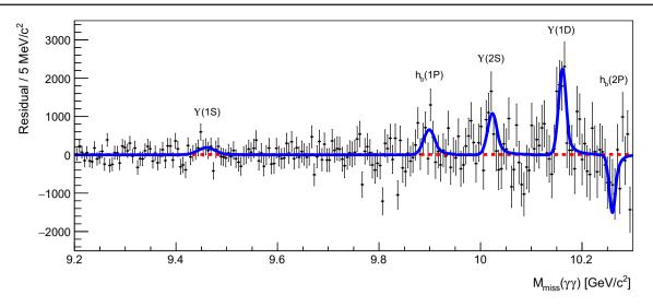
**Fig. 4**  $M_{\text{miss}}(\eta)$  distribution after the subtraction of the fitted background component. The blue solid line shows the signal component of the global fitting function, while the red dashed line represents the
