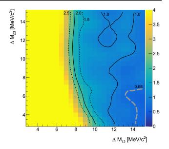
**Fig. 5** 90% C.L. upper limit on  $f_1$ , as function of the chosen  $\Upsilon_J(1D)$  fine splitting values. The black lines represent the curves at fixed values of the UL in steps of 0.5. The corresponding UL value is reported next to each line. Dashed and solid line styles are alternated for clarity. The thick gray dashed line demarcates the region excluded by the theoretically-favored value  $f_1 = 0.68$  [37]
