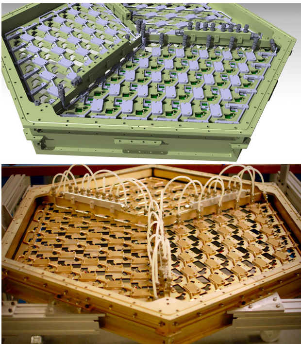
Fig. 26 Top a CAD drawing of the connection of the cooling pipes to the PDP backplate via aluminium blocks. Bottom a photograph of the backplate and pipes
